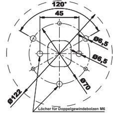
POSITION KLEMMRING IM ADAPTER / CLAMPING RING POSITION IN ADATER
